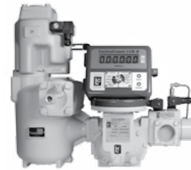
M7 Meter with LectroCount LCR-II Electronic Register, Optical Air Eliminator, High Capacity Strainer, and E-7 Valve
